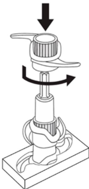
**Disassembling Tool for removing the upper and middle pair of blades**
